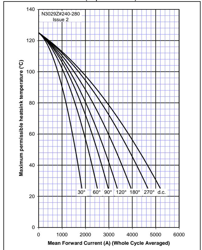
Figure 12 – On-state current vs. Power dissipation – Cathode Side Cooled (Sine wave)
