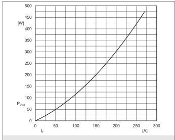
Fig. 1: Power dissipation per module vs. rms current
