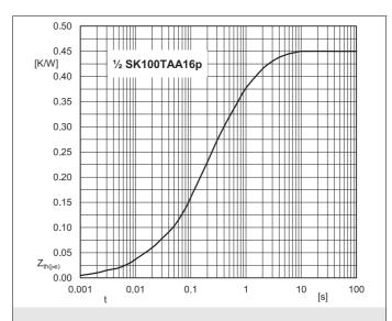
Fig. 2: Transient thermal impedance vs. time
