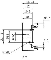
Suggested drilled hole diameter for terminal pins in the circuit board:
