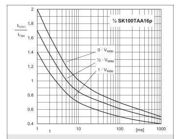
Fig. 4: Surge overload current vs. time
