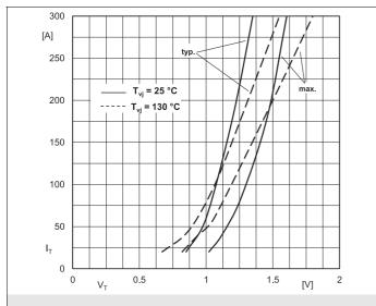
Fig. 3: Typ. forward characteristic of single thyristor
